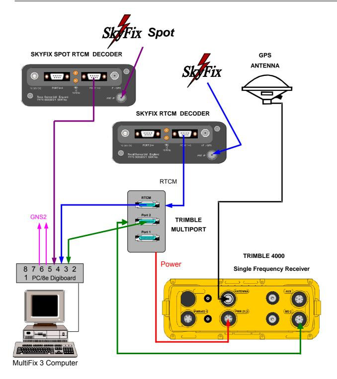
Typical MultiFix 3 Interconnection With Trimble 4000 GPS Receiver
