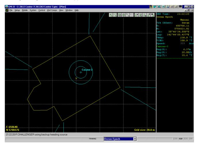
SkyFix Spot Differential GPS Position and Intended Position at the Casino-3 Location
