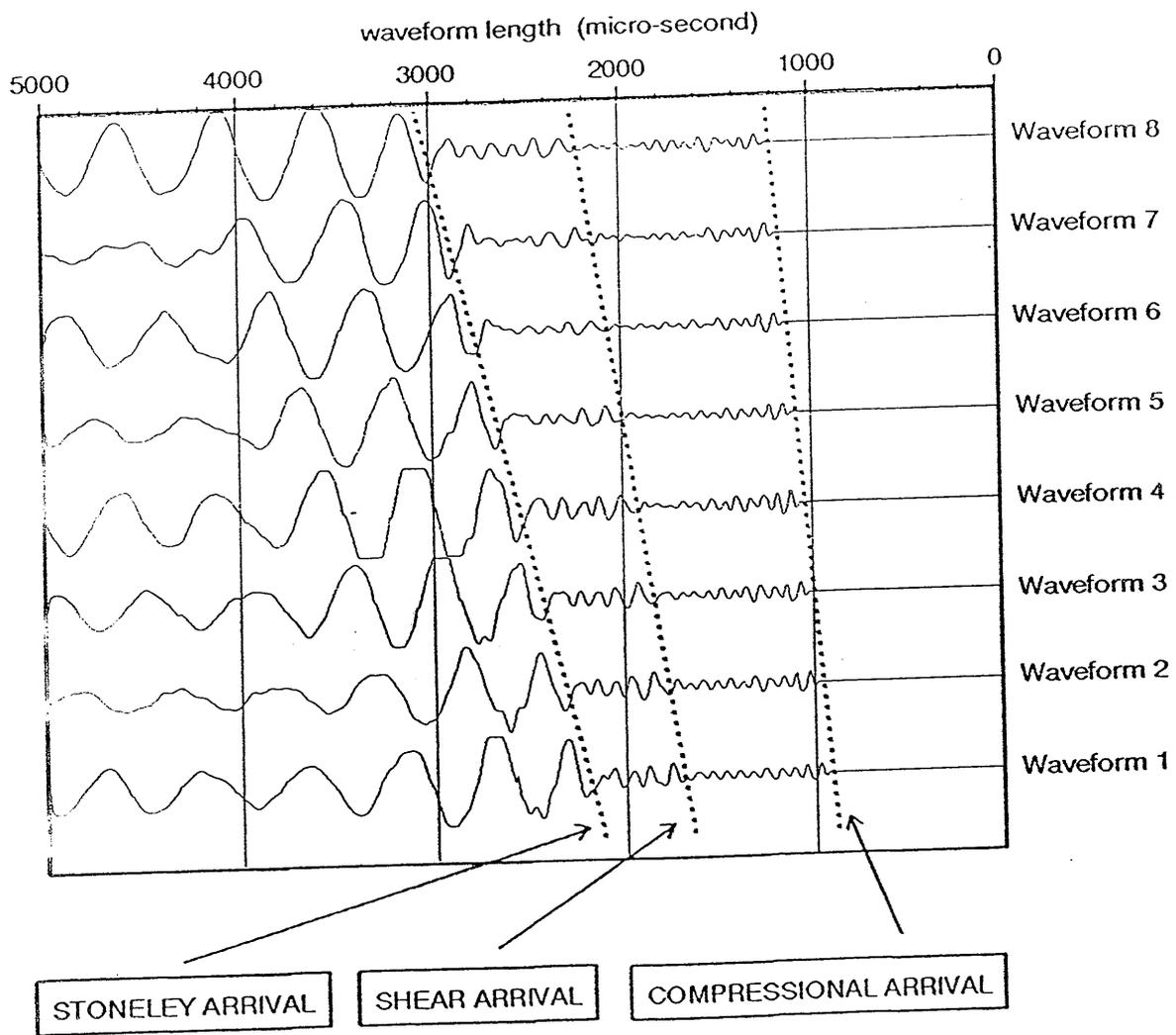
Figure 1 : Array Sonic Waveforms
