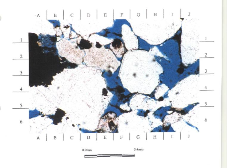
Figure 10. 1749.6m x75.6 PPL Massive quartz sandstone. Good primary porosity is evident (stained blue). Thin authigenic silica overgrowths can be seen at F2. The overgrowth can be seen to be coated with detrital clay.
