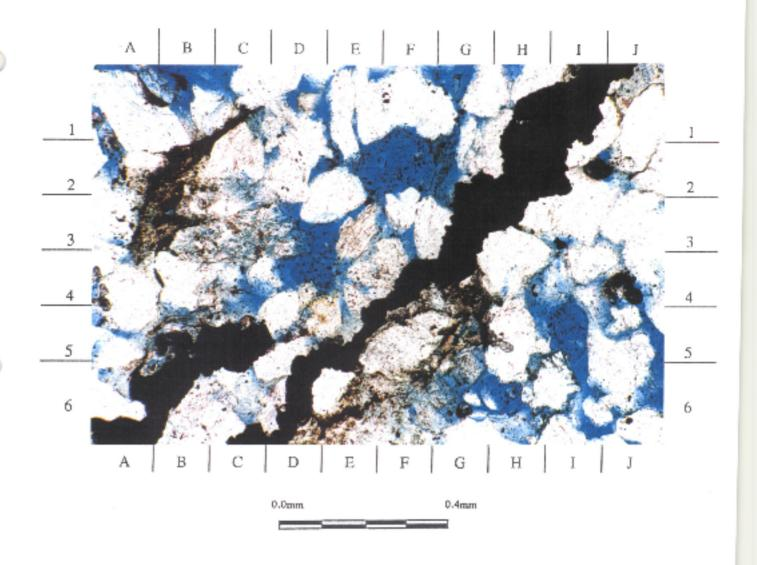
Figure 4. 1745.4m x75.6 PPL Good intergranular porosity (stained blue) is clearly evident. A pyrite lamination is visible running from J1 to D6, this can be seen to be associated with the brown detrital clays located at G4.
