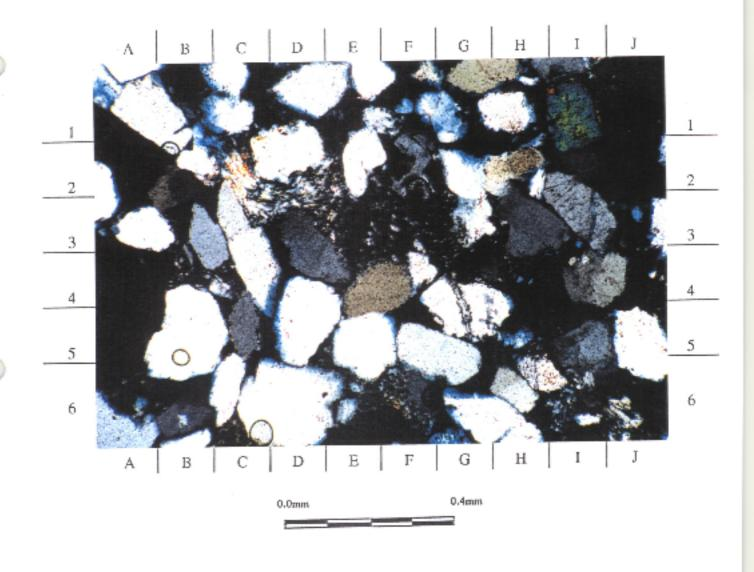
Figure 3. 1745.4m x75.6 XPL Quartz sandstone. A weak preferred alignment of the elongate axis of the detrital quartz is evident running from A1 to J1. A partially kaolinised muscovite grain can be seen at C2, with increasing kaolinisation to G3.
