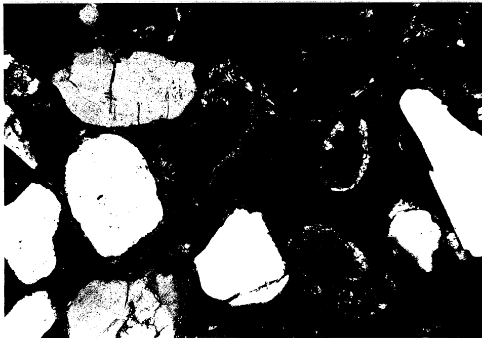
FIGURE 6 (a and b): Henke-1, SWC 9. PPL (a) and crossed Nicols (b), 2 mm. Typical field. Grains show a mantle of carbonate of several stages whereas most intergranular space is occupied by iron stained clay. Porosity (blue) is probably of secondary origin.
