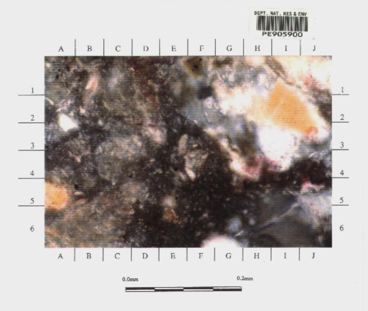
Figure 6. SWC 34 1465.7m x192 XPL Matrix material. The matrix appears to be composed of kaolinite, sericite and shattered volcanic fragments.
