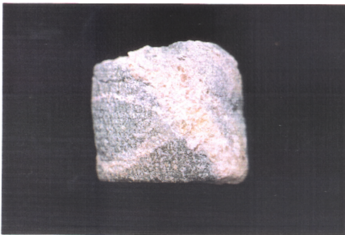
Detailed section of Core 4: Showing a dark greenish grey to mottled white, massive holocrystalline altered volcanic rock. The rock is sericitized, chloritized and contains quartz, mica, feldspars and amphibole. Calcite veins are common. The photo shows that many of the calcite veins displace earlier calcite veins.
