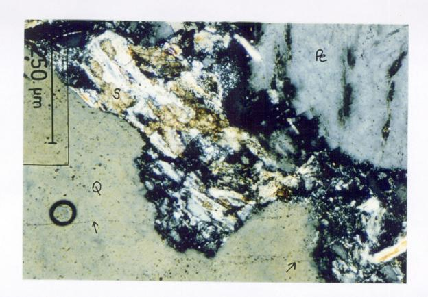
Figure 14 - Anemone #1A, junk sub sample, 4676a m. Carbonate spar (S) is corroding along cleavage of muscovite which is altering to grey chlorite. The quartz grain (Q) shows vacuole trails (arrowed) and inclusions. Dissolution is seen in the perthite grain (Pe).
