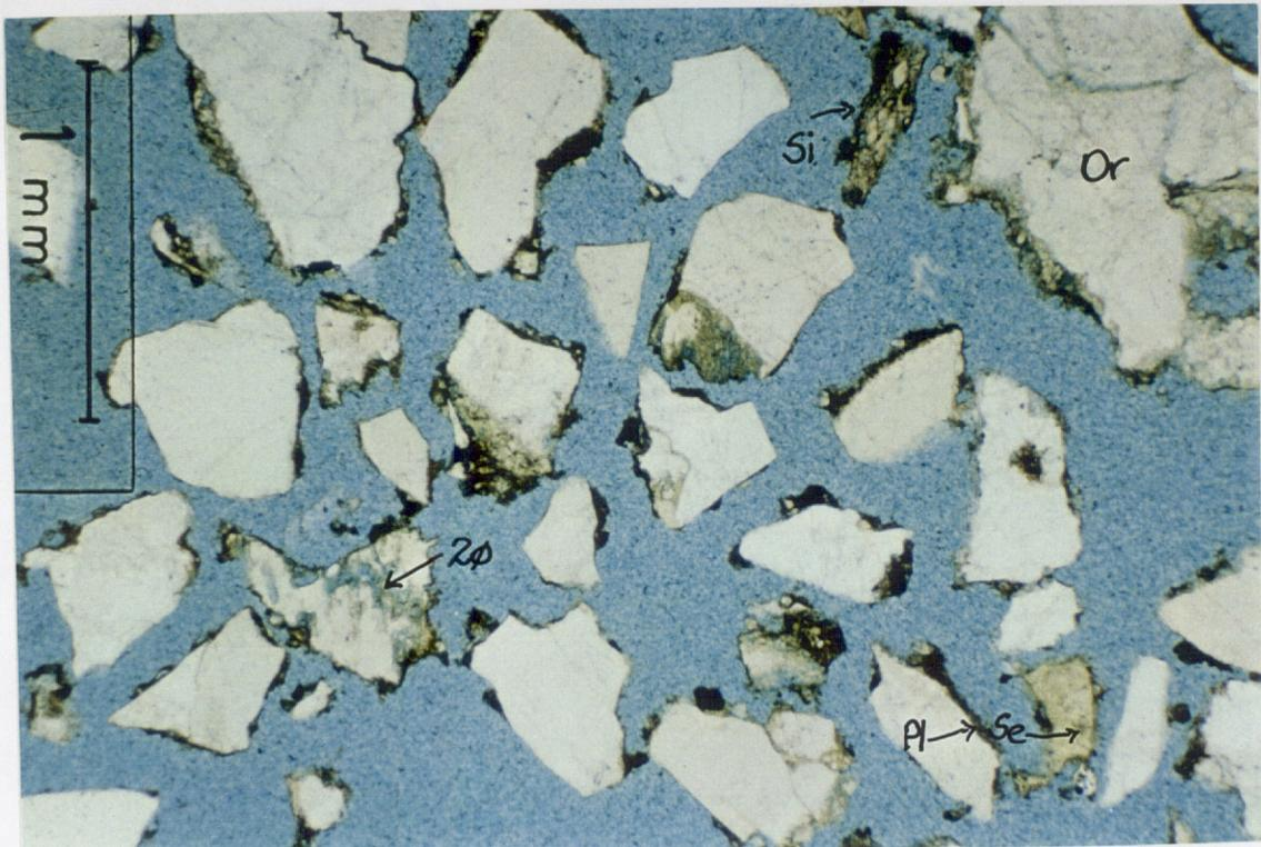
Figure 16 - Anemone #1A, cuttings, 4545 - 50m. (Plane polarized light). Chips from this sample show the plagioclase in perthite dissolving to create secondary porosity (2φ), orthoclase (Or) with a dusty, incipient sericite alteration and micritic siderite (Si) recrystallizing to sparry scalenohedra. Dark blobs of drilling mud glue small grains of quartz and feldspar and pyrite cubes to the larger chips.
