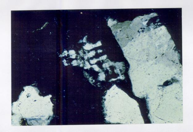
Figure #4 - Anemone #1, cuttings 4530 - 35m. The same field of view as Fig.3 under crossed polars shows hatched microcline twinning still showing in the skeletonized grain.
