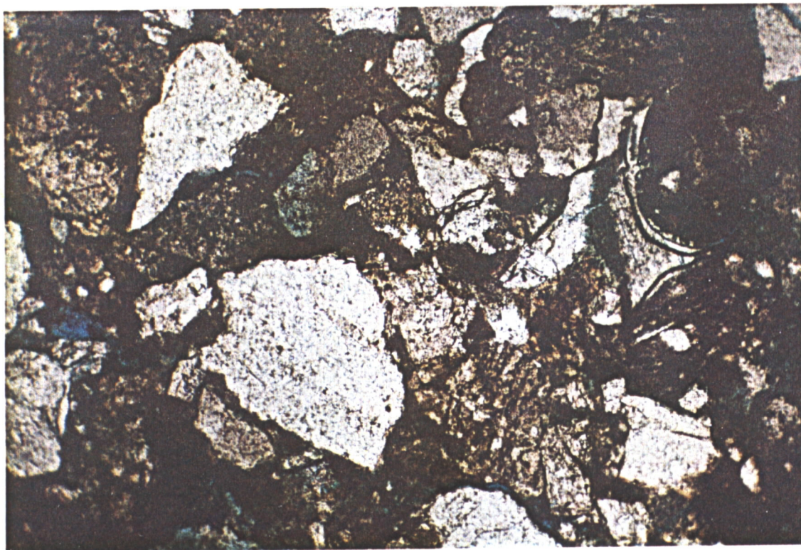
PHOTO 5 WIND. 2 1790M MODERATELY SORTED LITHIC ARKOSIC ARENITE. NIC UNC. FIELD WIDTH 1.8MM
