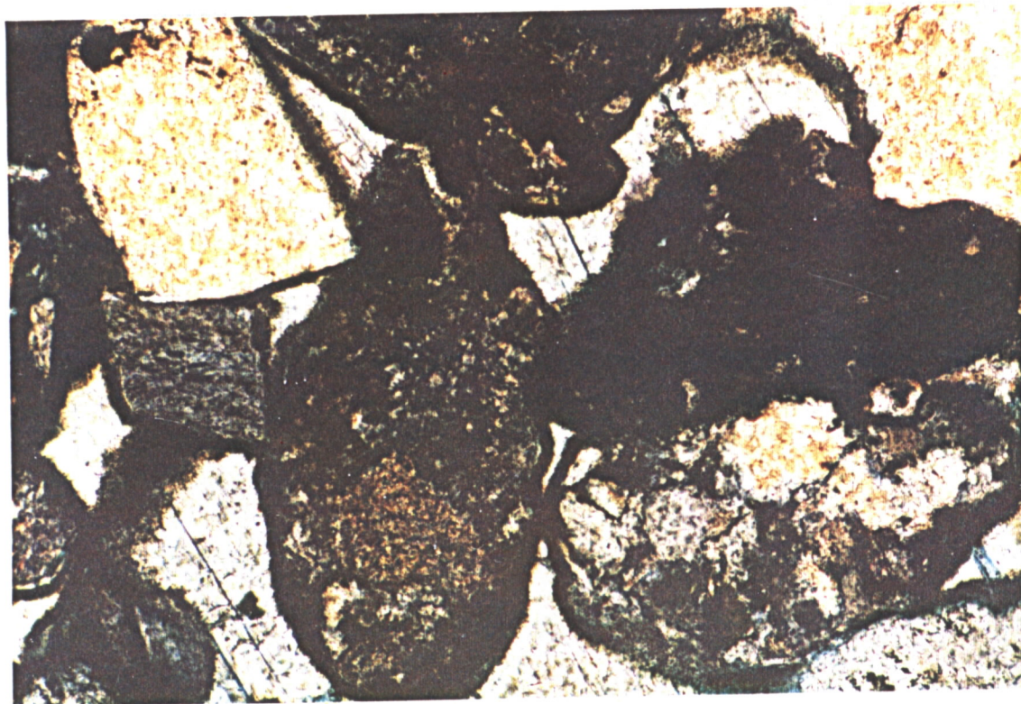
PHOTO 6 WIND. 2 1790M POIKILOTOPIC ?ZEOLITE CEMENT TO MIXED CLASTS. NIC CROS. FIELD WIDTH 0.7MM
