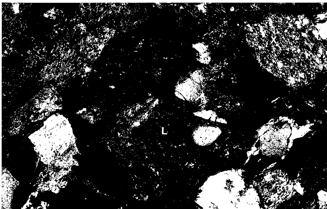
Figure 3: Sample 17: Plain light (upper) and cross-polarised (lower) photomicrograph of fine- to medium-grained, moderately sorted feldspathic litharenite. Photomicrograph shows abundant volcanic chert (L), sedimentary grains (X), pyrite (P) and detrital clay matrix (M). Long axis of photomicrographs is 1.25mm.
