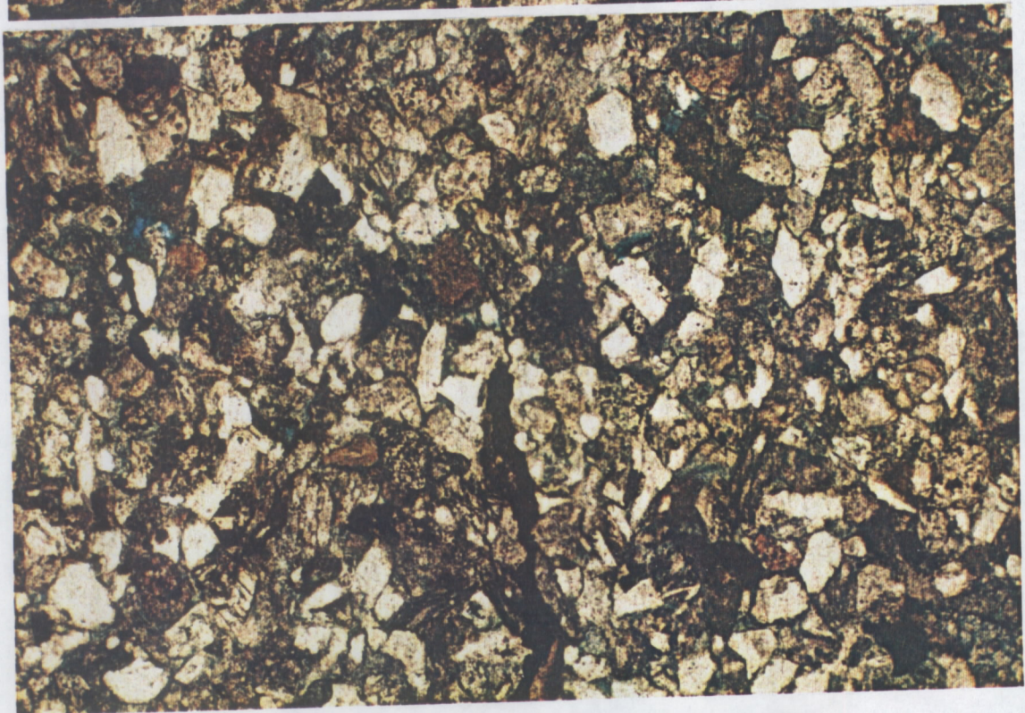
PHOTO 4 P.CAMPBELL 4 CORE 26 8279-8299FT WELL SORTED TUFFACEOUS SANDSTONE WITH CARBONACEOUS STRIP. NIC UNC. FIELD WIDTH 1.8MM.
