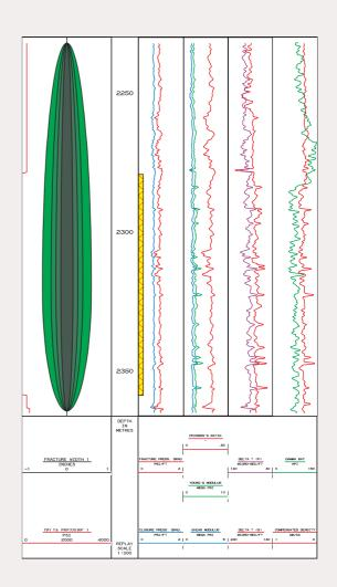
Behind Casing Velocity Analysis (BCV left) generates formation slowness (inverse velocity) logs in cased wells. The algorithm windows LCS waveforms and searches for coherent arrivals across the receiver array. Velocities are picked from a semblagram that indicates the degree of waveform similarity as a function of moveout and depth. The semblagram also provides quality control across poorly bonded intervals where formation signals are weak.
