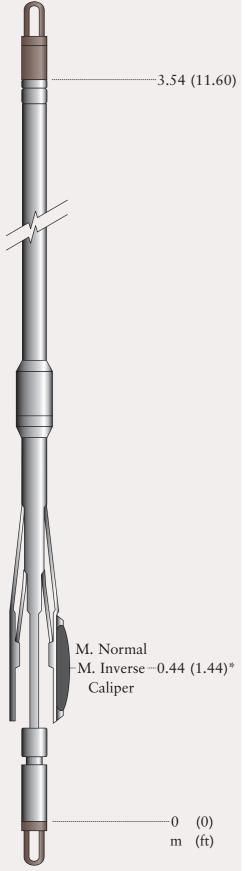
\* Caliper depth offset calculated at 200 mm (7.9 ins) diameter
