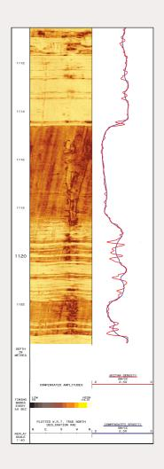
Upper left : Compensated Density and VECTAR high resolution density with an AST amplitude image.
