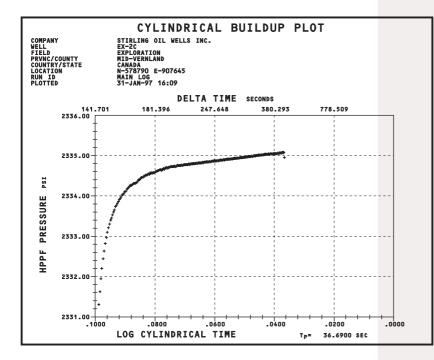
RFS pressure-time function plots are used to compute intrinsic formation pressures and to provide estimates of formation permeability. During acquisition, tests are terminated as soon as the computed formation pressures reach steady values - this can greatly reduce total logging times.
