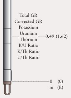
The **Two Arm Caliper** measures borehole diameter without exerting eccentralisation forces. As such, it is commonly used with oriented density tools to provide an orthogonal X-Y caliper pair. In oval holes this allows confirmation that the density shoe is correctly positioned across the short axis of the hole (for optimum shoe contact). The X-Y combination also provides a more accurate determination of hole volume.
