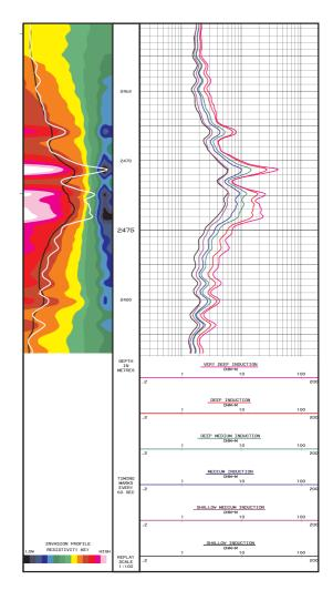
**VECTAR**<sup>©</sup> acquisition and processing enhances the resolution of many conventional logs by between 50 and 300 %, giving improved bed definition, core correlations and nett pay results in thinly bedded and complex reservoirs.
