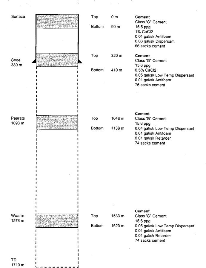
Mix Water After Plug Displacement
