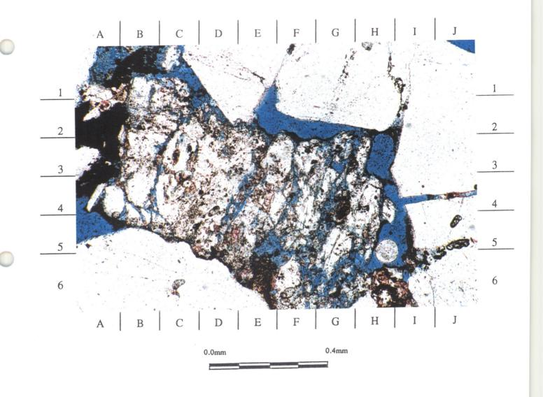
Figure 5. 1746.3m x75.6 PPL Quartz sandstone with good intergranular porosity (stained blue). Secondary porosity is also evident within the heavily leached feldspar at F4. Thin detrital clays are also visible coating the primary pore space at H3.
