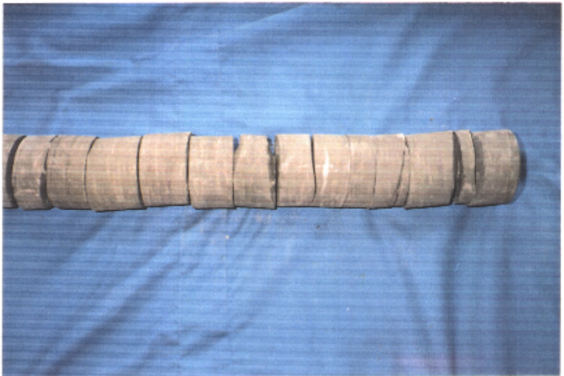
Section of Core 3 (1785.2 - 1790.1m): Pretty Hill Formation - Crayfish Subgroup. A typical section of core at this level. The rock is extremely friable siltstone and the core has fractured apart at regular intervals. Frequent laminae of light grey sandstone exist here with resultant flame structures evident throughout the core. Cross bedding and erosional surfaces can be observed, along with sections of more massive unfeatured siltstone.
