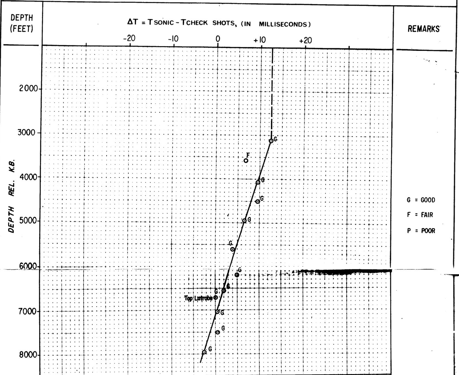
$$\text{Slope} = \frac{\Delta T_2 - \Delta T_1}{D_2 - D_1} = \frac{(-2.4) - 12.3}{7955 - 3124} \times 1000 = -3.04 \mu\text{sec./ft}$$
