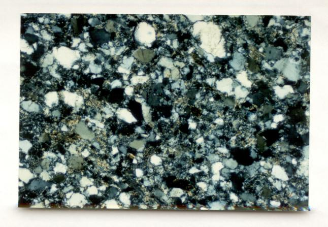
Figure 15: SWC 58, 2294m, 2mm, CL A typical field-of-view in very fine-grained sandstone.
