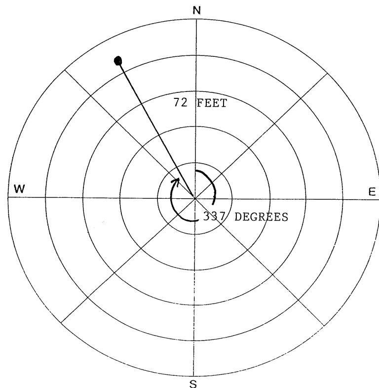
INDICATE GUN/VIBRO AND HYDROPHONE OFFSET AND AZIMUTH RELATIVE TO NORTH
