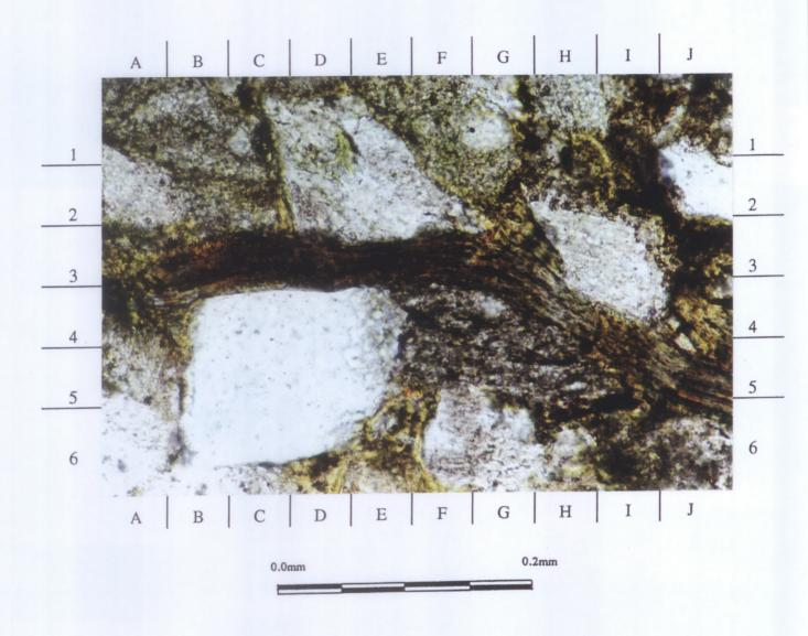
Figure 5: 7895'-7897' x192 PPL. Lithic rock with a detrital biotite grain at A3-J5. Partial chloritisation of the detrital biotite is evident. Authigenic chlorite is also evident along the margins of the framework grains.
