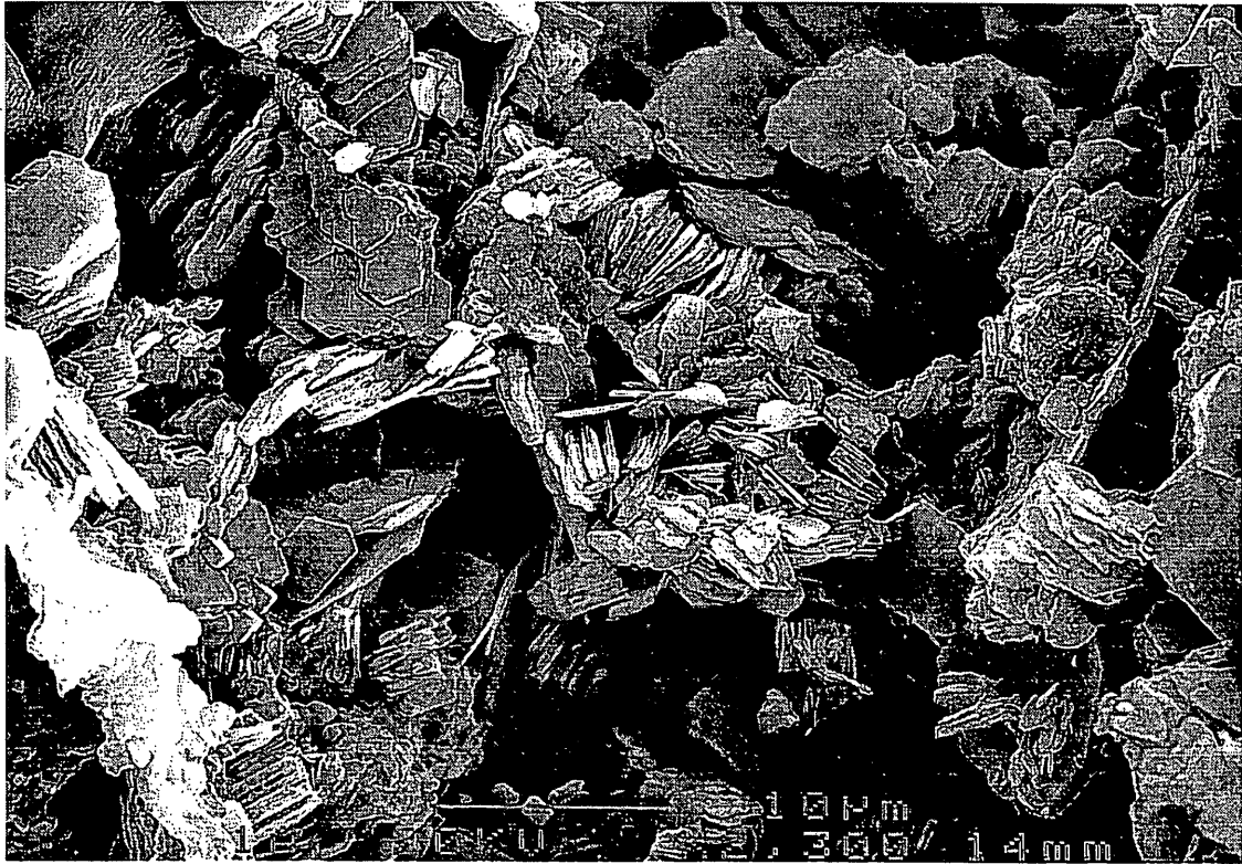
Plate 16: Sample # 1 (1509.67 m): SEM photomicrograph showing abundant kaolinite cement. Kaolinite occurs as pore filling around highly altered lithic fragments and mica flakes. Kaolinite occurs as hexagonal platelets forming short booklets. Note microporosity between kaolinite cemented areas. Scale bar = 10 \mu\text{m} .
