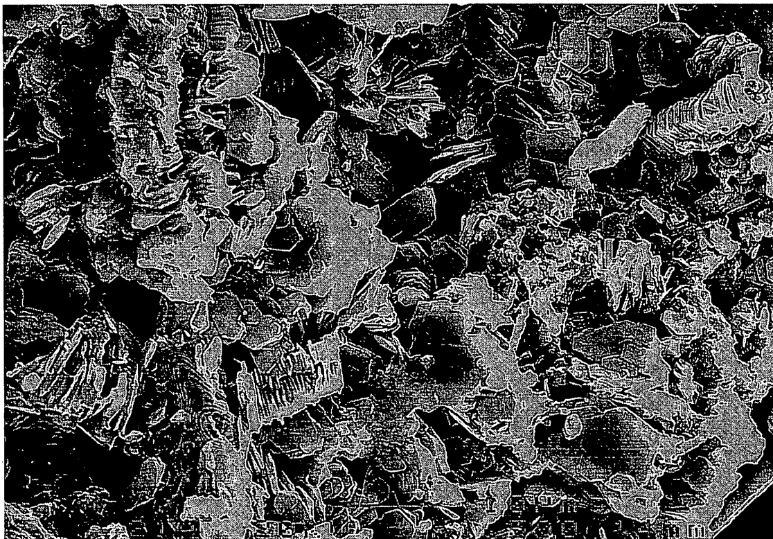
Plate 26: Sample # 21 (1529.60 m): SEM photomicrograph showing authigenic kaolinite around altered ductile lithic grains and mica flakes. Authigenic kaolinite occurs as randomly oriented pseudo-hexagonal, vermiform and book-like species and occupies few of the intergranular pore spaces. Scale bar = 10 \mu\text{m} .
