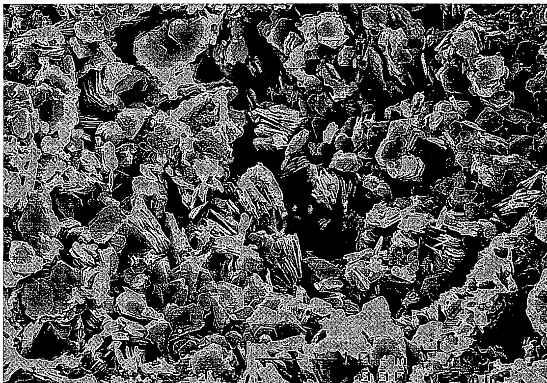
Plate: 20: Sample # 9 (1527.77 m): SEM photomicrograph showing kaolinite booklets filling the pore spaces. Kaolinite crystals occurs as pseudohexagonal and book-like crystals developed face to face. Scale bar = 10 \mu\text{m} .
