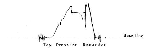
DRILL STEM TEST Nº4, 5774'- 6005' (schlumberger) 5/8''bottom choke, no water cushion, immediate strong blow decreasing to weak blow in 45 min., dead in 1hr., recovered 900' drilling mud and 4600' formation water (15,950 ppm NaCl)
