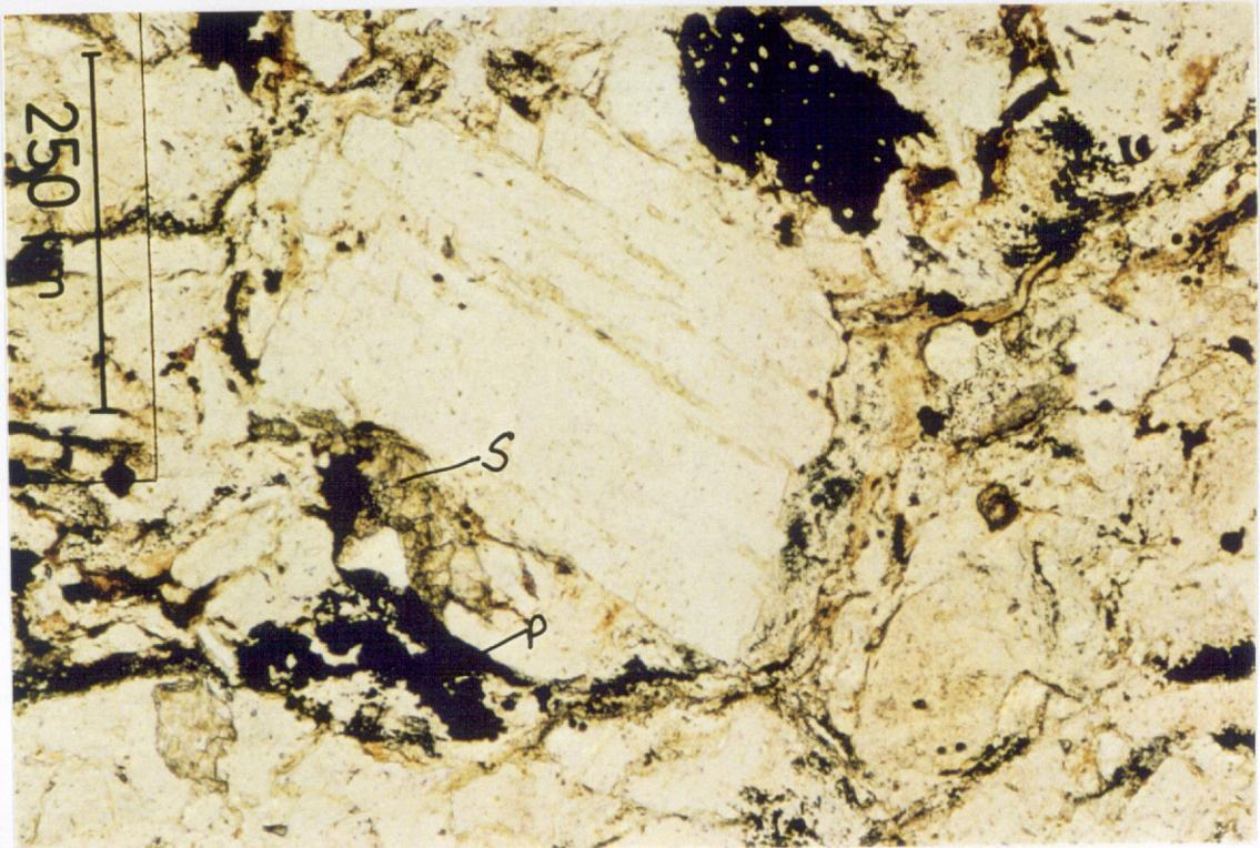
Figure 11 - Anemone #1A, junk sub sample, 4676a m. The central feldspar cleavage fragment shows alteration along cleavage in plane polarized light. Carbonate spar (S) is mildly corroding the feldspar. A structured organic fragment (?wood) occurs at the top right of the field of view and an aggregate of pyrite crystals (P) is visible.
