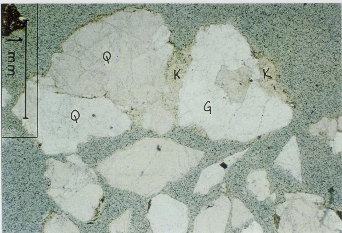
Figure 6 - Anemone #1A, cuttings 4530 - 35m. (Plane polarized light). A composite of sediment grains is cemented by pore-filling kaolin (K). The grains of the composite are quartz (Q) and a granite fragment (G) with a perthite grain in the centre. Some fine sand and clay matrix is attached to the chip in the lower left.
