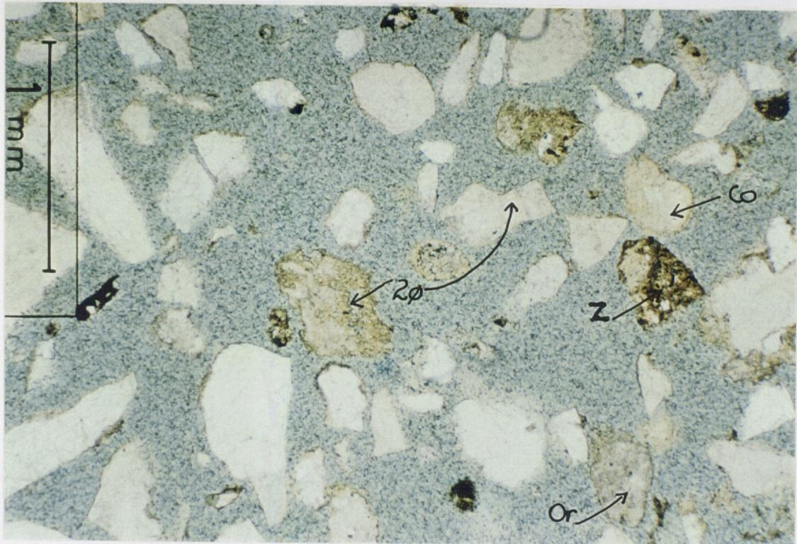
Figure 1, Anemone #1A, cuttings, 4530 - 35m. (plane polarized light). Crushed grains from the washed sample show quartz as clear grains, orthoclase with dusty sericite alteration (Or), a composite grain or very fine sandstone (Co) and an organic rich siltstone (Z). Two grains of microcline show dissolution to form secondary porosity (2ø).
