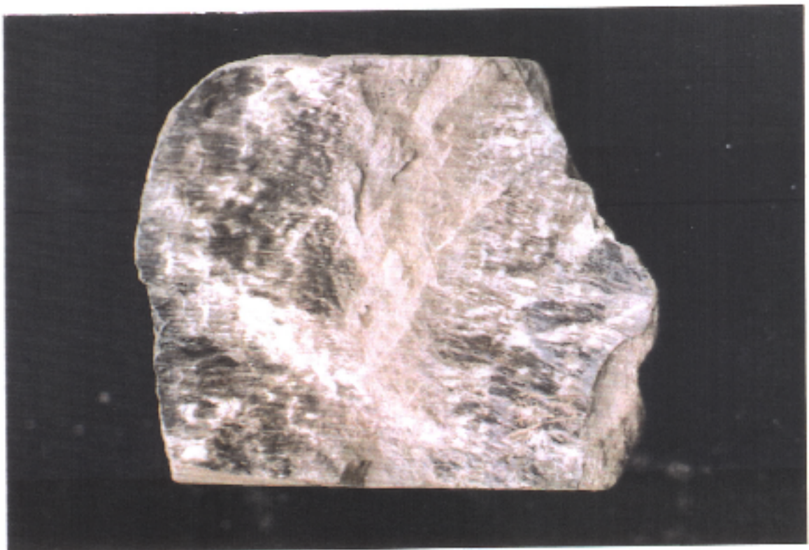
Section of Core 2: Shown is a vertical slickenside surface near the base of the core.
