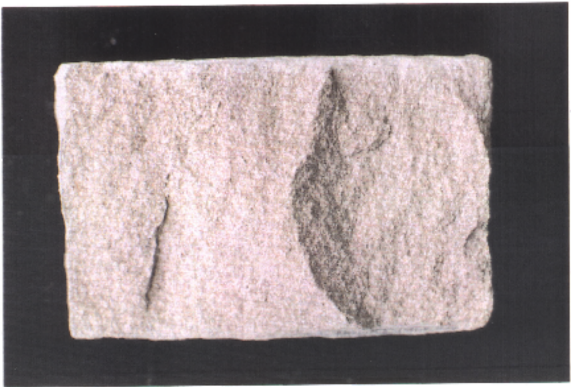
Detailed section of Core 2: Showing a vertical cross section through an upper part of the core. The sandstone is light grey, massive, quartzose and well sorted. Also present is trace silica cement, trace calcite cement, argillaceous matrix and common lithic grains and garnets. The core has low visual porosity.
