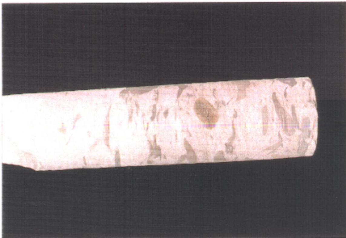
Section of Core 2 (1509.8 - 1515.8m): Pretty Hill Formation - Crayfish Subgroup. Continuous section showing the transition from the upper massive sandstone with occasional clay lenses to a sandstone with occasional, increasing to common claystone clasts. There are no obvious bedding features, although clast orientation suggests horizontal bedding.
