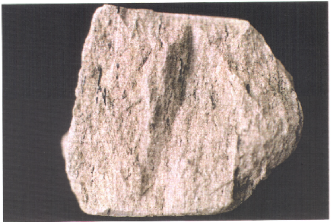
Detailed section of Core 1: Showing carbonaceous specks and plant/ coally material in claystone in the basal part of the core. Olive grey to light olive grey, argillaceous, non calcareous, micaceous, occasionally laminated.
