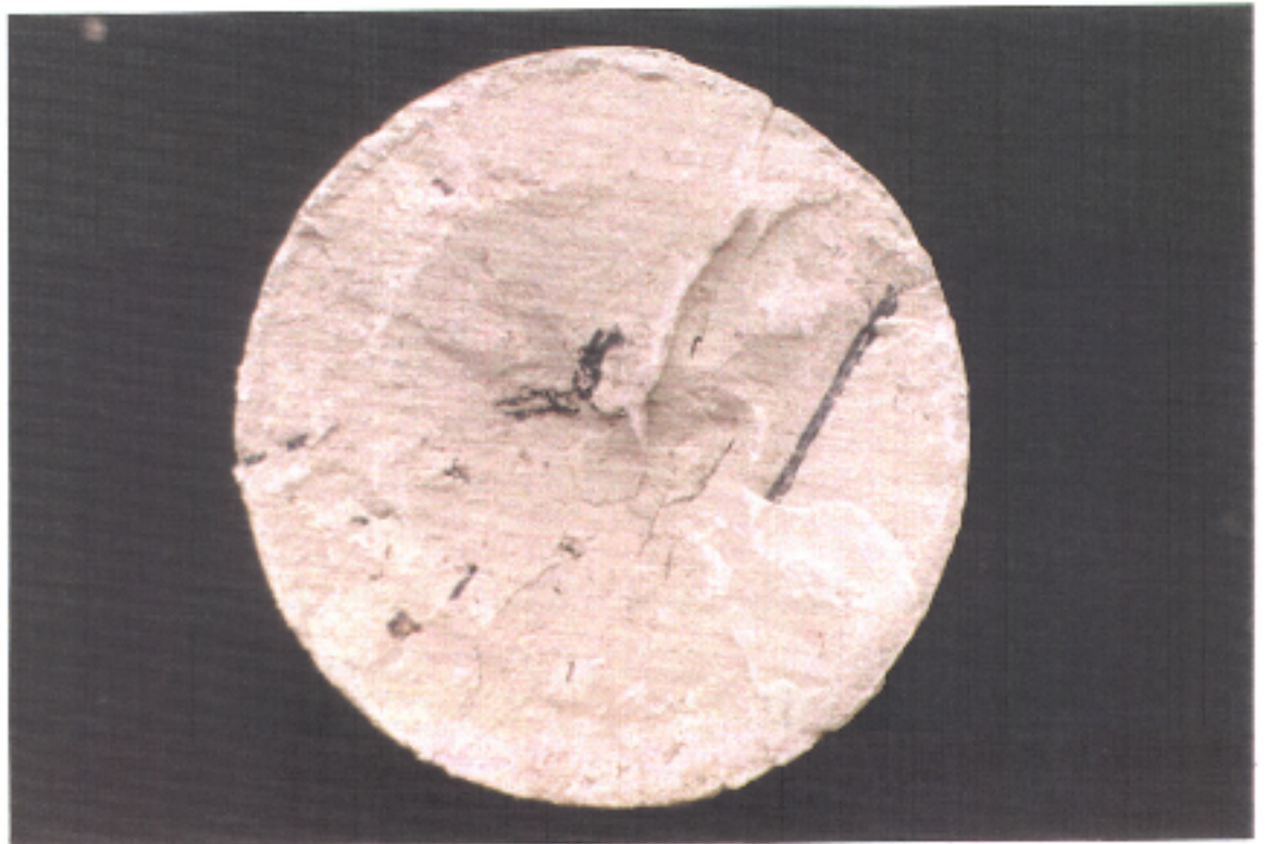
Top of Section of Core 1: This slice through the top of core 1 shows well preserved plant material embedded in massive claystone.
