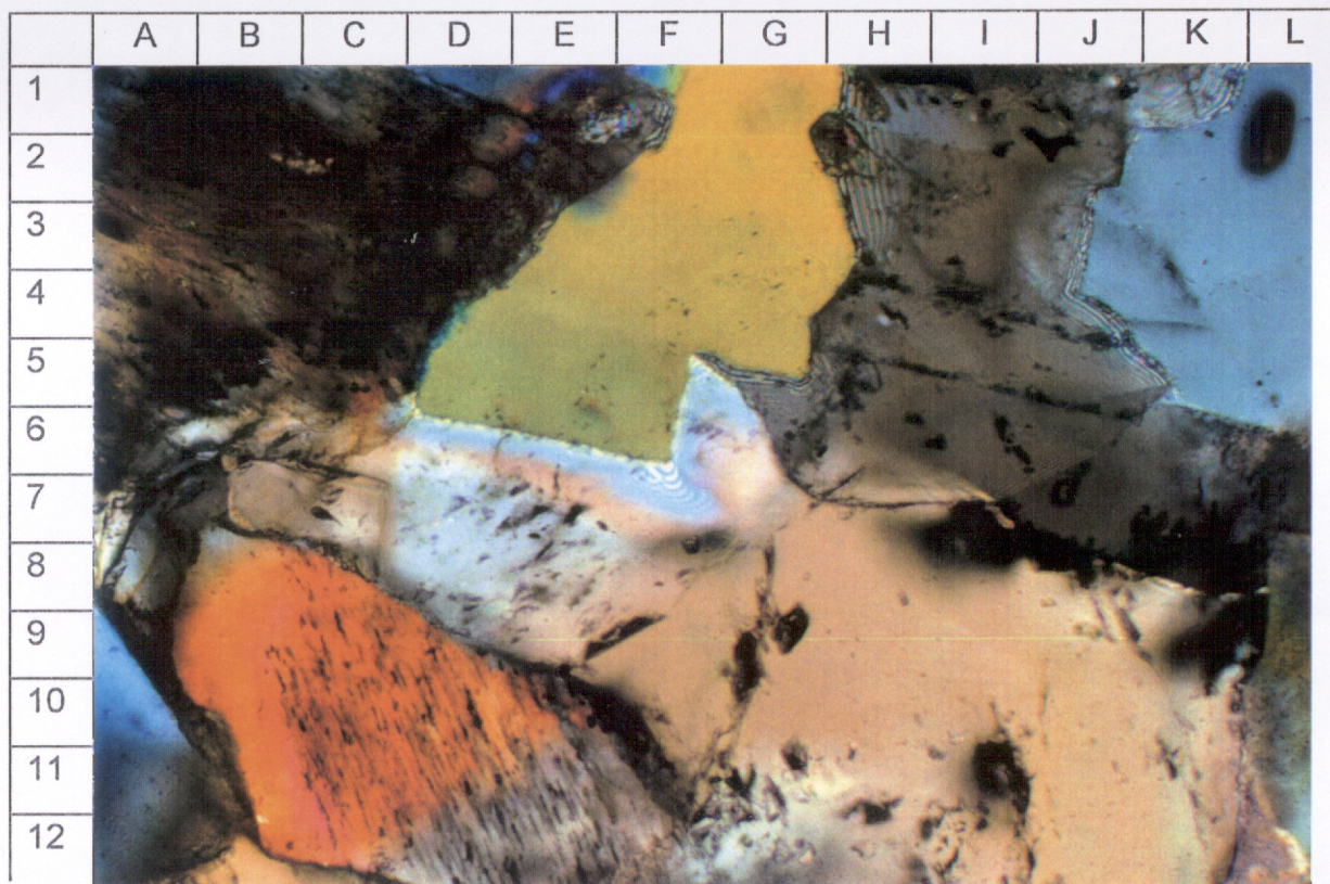
Figure 1B Replacement of labile grains by mixed layer (illite-smectite) clays (e.g. J:5). Veilfin-1, 3370-75 m cuttings sample, transmitted light with cross nicol (100 \mu\text{m} = 17.5 mm).
