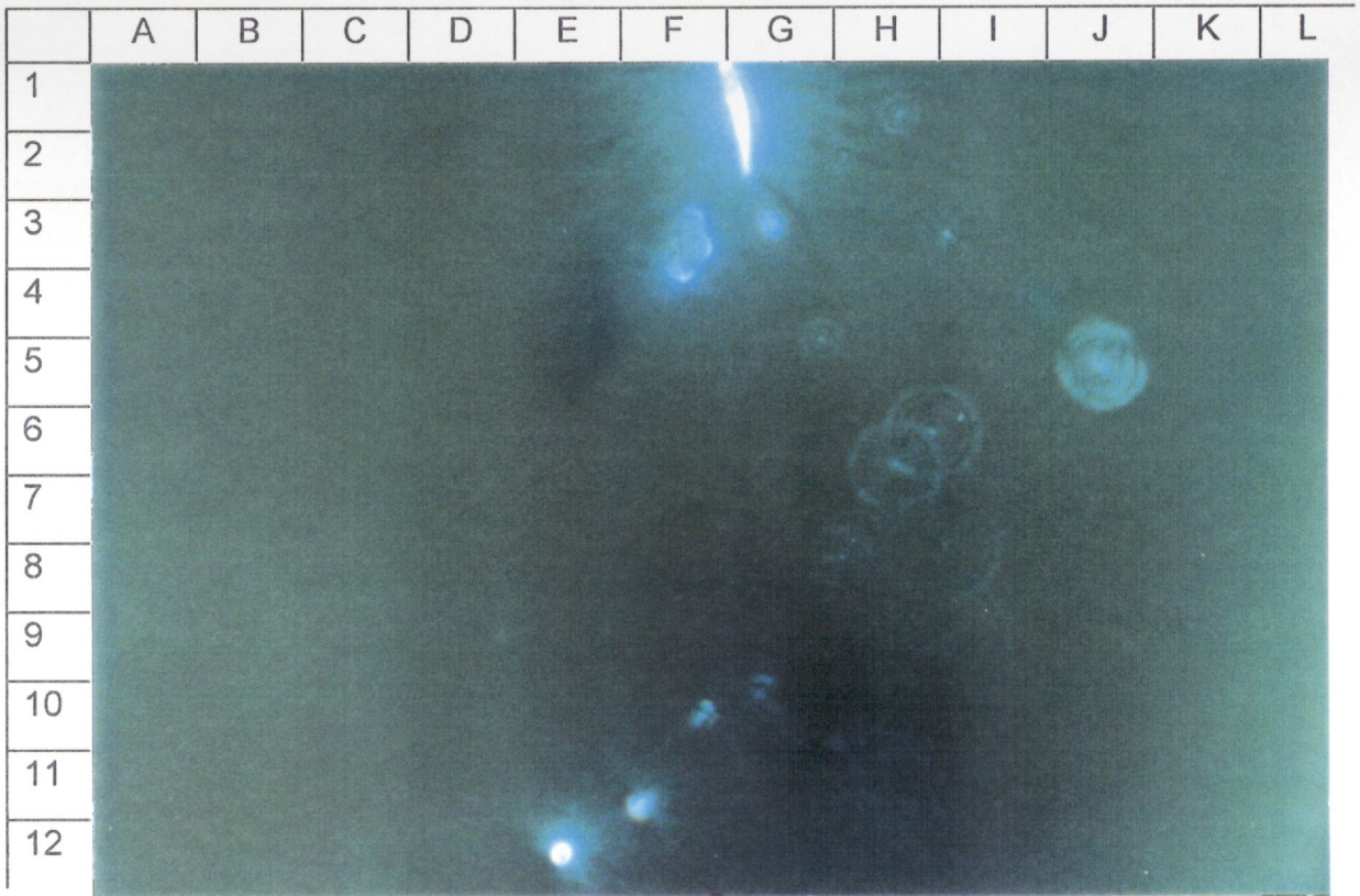
Figure 6B Same subject as 6A taken in transmitted light. Note the low refractive index of the dark gas bubble in the inclusion at F:3. Inclusions containing mostly gas could either represent condensate or mixing of oil and gas.
