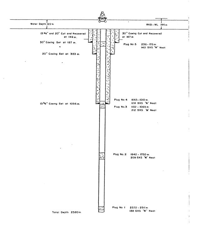
When the weather died down, the stack and riser were pulled. The  $16\frac{3}{4}$ " wellhead housing was latched into and an attempt to pull all three casings was made. The  $16\frac{3}{4}$ " wellhead with the 20" casing stub and the  $13\frac{3}{8}$ " casing stub inside were recovered. Several attempts were made to relatch into the 30" housing, all unsuccessful.
