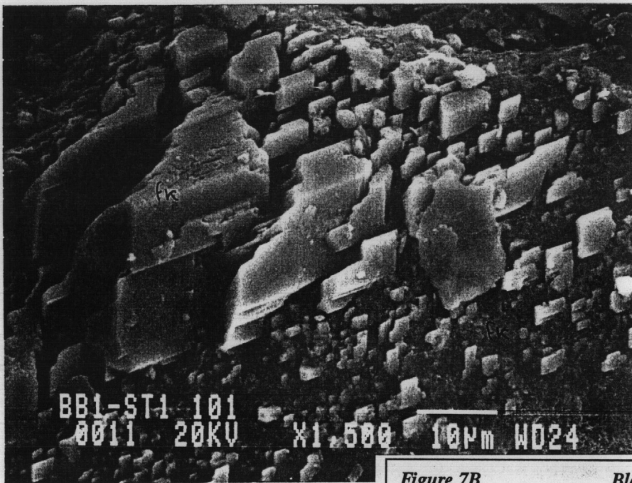
Figure 7B Blackback 1 ST 2917m K-Feldspar overgrowths on K-Feldspar detrital grain. Cryptocrystalline micro porous chert grain.
