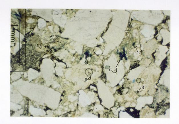
Figure 16. Anemone #1A, junk sub sample, 4676b m. Thin section micrograph in plane polarized light demonstrating areas of secondary dissolution porosity (d) and fracture porosity (f). Microporosity may well be present. The stylolitic nature of organic matter (and opaques?) is evident. At the left of the photo is a concentration of spar crystals (S).
